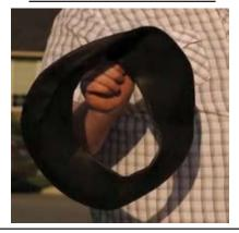
Helpful Hit: The tire should be loose and separated from the rim as shown in the image below.
