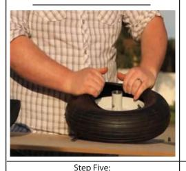
Line up the valve stem with the valve hole on the rim. Put the new tube in your tire by working your way around the tire openng. Press the tube up against the edge of the tire as you install it. Pull the valve stem through the valve stem hole in your rim.
