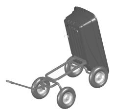
Chock the wheels. Rotate the Wire Latch so it is unlocked. Place your hands under the lip on the Flat End of the Sled. This lip will allow you to easily pivot the Sled upwards, dumping the contents. The Pointed End of the Sled will touch the ground when it is in the full dump position.
